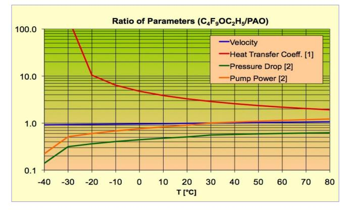
Note: Flow calculations for 3M Novec<sup>™</sup> 7200 (HFE) versus Polyalphaolefin (PAO). (1) Higher HTC is better; (2) A lower pressure drop value is better and a lower pump power requirement is better. Source: 3M Company.
